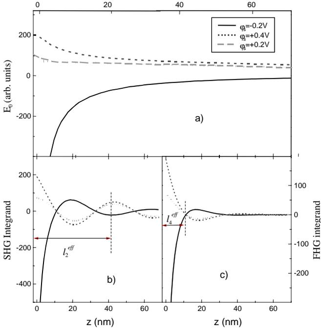
**Fig. 6.** **a** Spatial distribution of DC-electric-field for Si/SiO<sub>2</sub> MOS structure (n-type,  $N_D = 10^{17} \text{ cm}^{-3}$ ) for various surface potentials; **b, c** spatial distribution of integrand in (10) for **b** SH, and **c** FH
