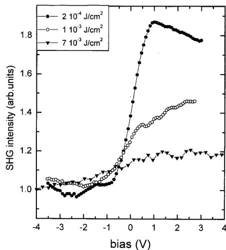
**Fig. 4.** EFISH dependences measured at various fluences of fundamental radiation
