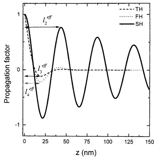
Fig. 5. Propagation functions for SH, TH and FH waves in silicon at 800 nm fundamental wavelength
